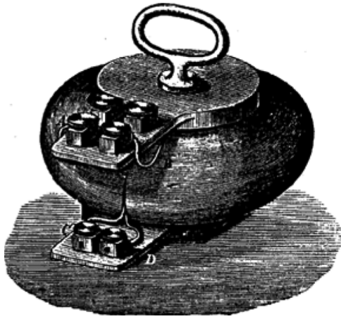
Fig. 2. Drawing of the Ganz factory transformer [2].
